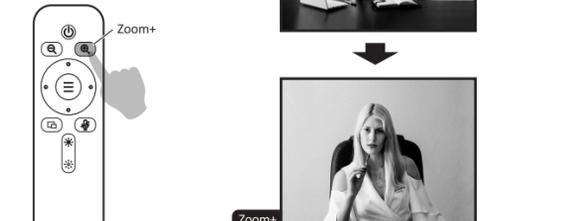
After the image is zoomed in, press Up /Down / Left / Right to move pan and tilt to control EPTZ.
